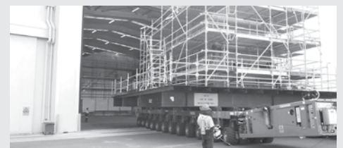
Moving: Block 715 moving into the Blast and Paint Chamber.
