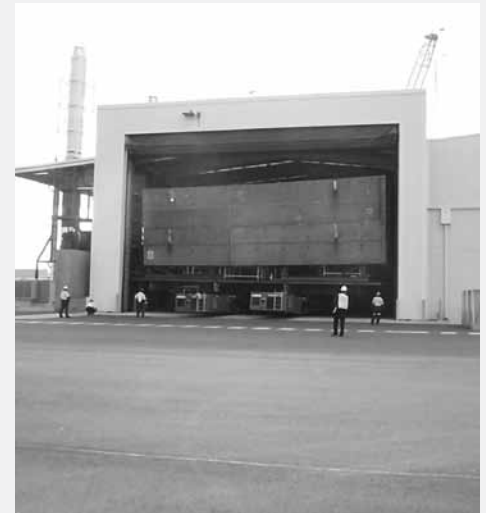
Movement: Block 409 moving into the Blast and Paint Facility.
